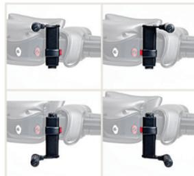
Shown above are the two arm support holders in the four positions possible. Arm support holders can be placed on either side of the body support, with the post forward and up, forward and down, rearward and up, or rearward and down, giving a wide range of adjustment.
