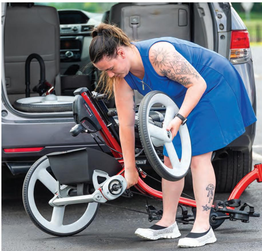
Remove rear wheels and front end, and flip down the backrest for easy transport.
