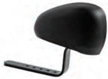
**Abductor:** The abductor separates the knees and helps to control spasticity that causes leg scissoring. The abductor can be adjusted forward and back in three positions.
