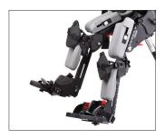
Advanced legs have independent leg length, hip angle and knee angle adjustments.
